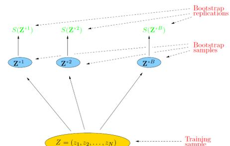
**FIGURE 7.12.** Schematic of the bootstrap process. We wish to assess the statistical accuracy of a quantity  $S(\mathbf{Z})$  computed from our dataset.  $B$  training sets  $\mathbf{Z}^b$ ,  $b = 1, \dots, B$  each of size  $N$  are drawn with replacement from the original dataset. The quantity of interest  $S(\mathbf{Z})$  is computed from each bootstrap training set, and the values  $S(\mathbf{Z}^1), \dots, S(\mathbf{Z}^B)$  are used to assess the statistical accuracy of  $S(\mathbf{Z})$ .
